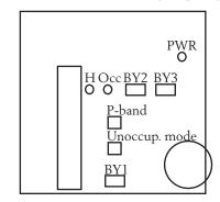
Jumper BY1 Right = Internal sensor (factory setting)
