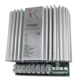
CTR25 is a 3-phase controller intended for time-proportional control of electric heaters, radiators, etc. The controller is capable of controlling both D- and Y-connected loads.
