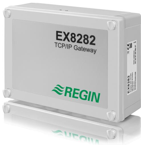
*Communication gateway for TCP/IP communication, intended for connecting one or several controllers with serial communication to a computer network.*
