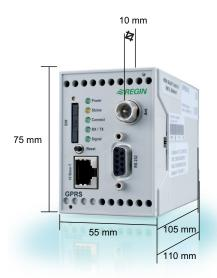
The cabinet should have a depth of at least 155 mm for the antenna to fit without bending the cable too much.
