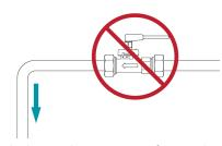
Figure D:straight downwards pipe can cause flow rate discontinuity.
