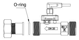
It is important to verify the maximum torque applied to the hexagon of the device because the plastic body of the flow meter can be damaged.
