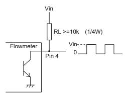
Notathe frequency output is a square wave with 50% duty oscillating between Vin (positive power supply) and ground. The frequency is available on Pin 4, an external resistor must be mounted between Pins 4 and 1 (RL  $\geq$  10 k $\Omega$  Q1/4 W).
