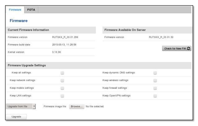
**Keep settings** – if the check box is selected router will keep saved user configuration settings after firmware upgrade. When check box is not selected all router settings will be restored to factory defaults after firmware upgrade. When upgrading firmware, you can choose settings that you wish to keep after the upgrade. This function is useful when firmware is being upgraded via Internet (remotely) and you must not lose connection to the router afterwards.
