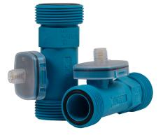
Flow-meter is a direct type of flow-measuring device with operating fundamentals based on the Von Karman principle. A piezo-elettric sensor detects the vortices, which are converted into an electrical frequency signal.
