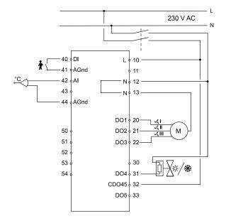
Wiring diagram for thermal actuator
