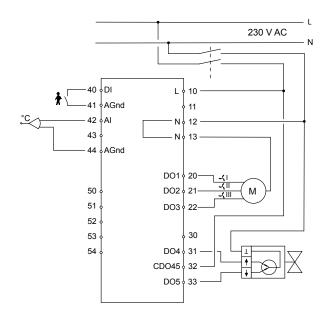
Wiring diagram for 3-point actuator
