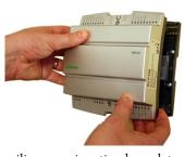
The modular design with a separate bottom plate for wiring makes the unit easy to install and commission. The bottom plate can be put into place before the electronics are installed.
