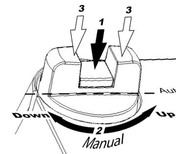
To manually set the valve position, first depress the central part of the knob until it clicks in place and remains depressed (1 in the figure). The valve position may then be changed manually by turning the knob (2 in the figure). Clockwise rotation will extend the drive rod and anti-clockwise rotation will retract it.
