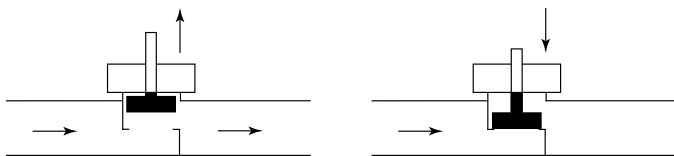
Figure 3 Left: Valve is open when the valve stem is extended. Right: Valve is closed when the valve stem is pushed into the valve.
