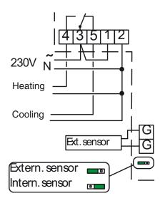
**NB:** The thermostat may control either heating or cooling, but not both simultaneously.
