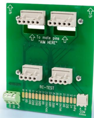
In order to make measurements and test the inputs/outputs of a Regio room controller during installation, Regio's RC-TEST service adapter may be used.
