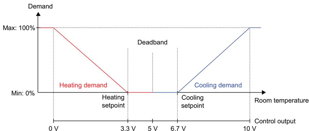
Figure 3-45 Simplified view of an AO configured for the 6-way valve with the controller in controller mode Heating + Cooling + VAV
