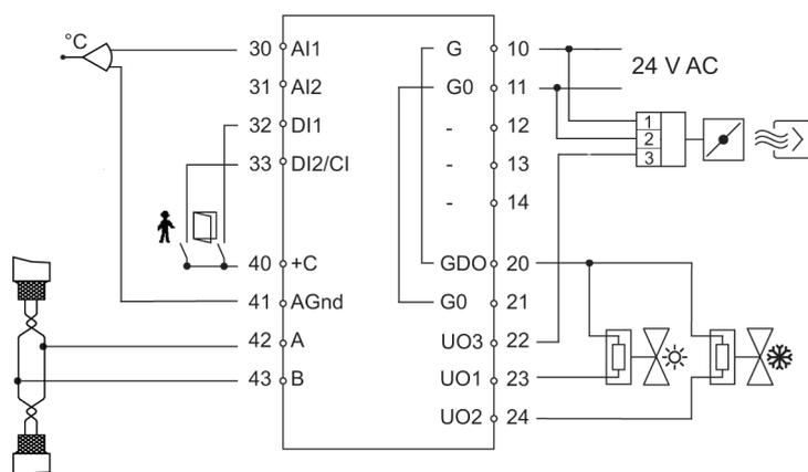
Figure 6-4 Connection diagrams for model with built-in CO<sub>2</sub> sensor.
