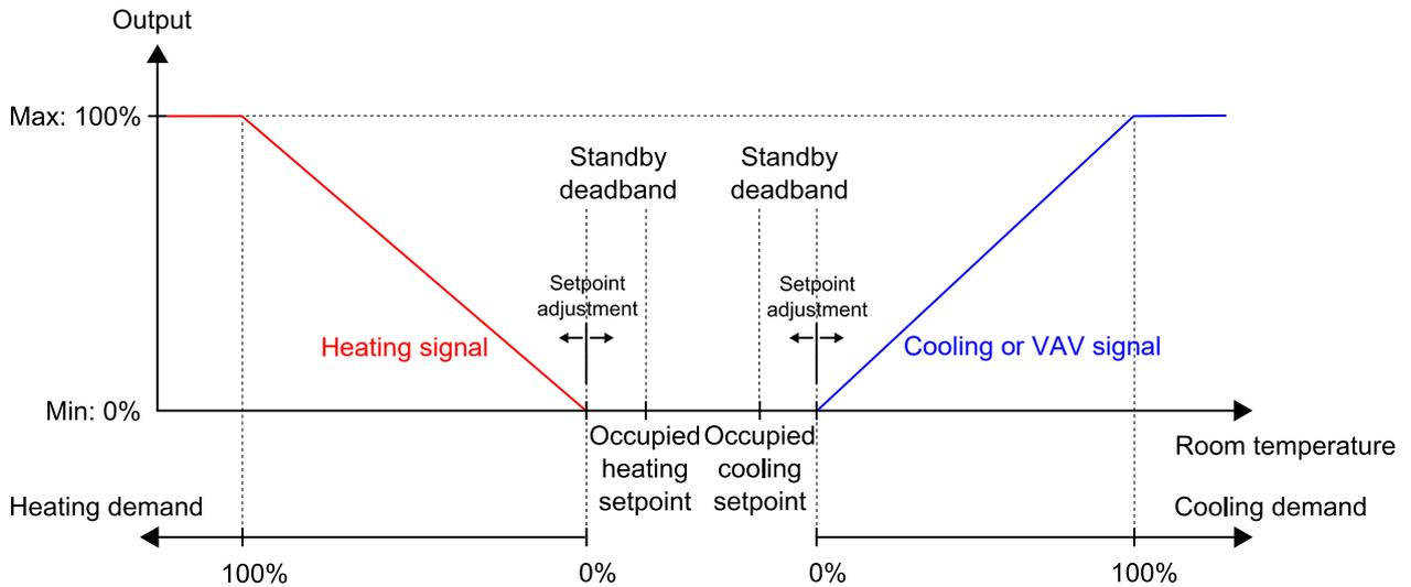
Figure 3-27 Control behaviour for the standby controller state.
