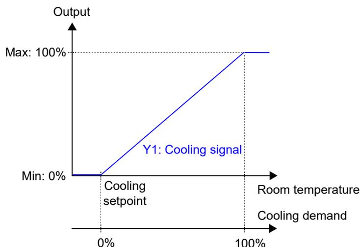
Figure 3-5 Control behaviour for the Cooling controller mode.
