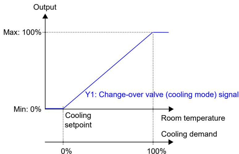
Figure 3-15 Control behaviour for the Heating/Cooling (change-over) controller mode when the controller is in cooling mode.
