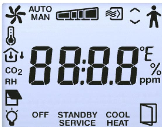
Figure 4-4 Indications in controller display.
