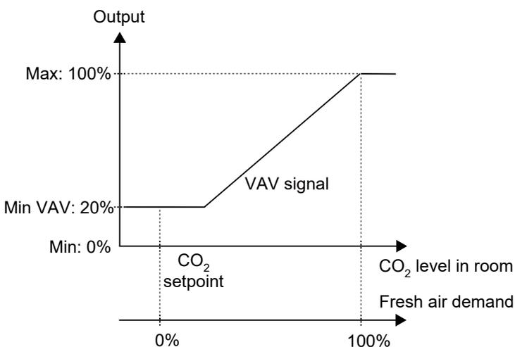
*Figure 3-44 CO<sub>2</sub> control behaviour.*
