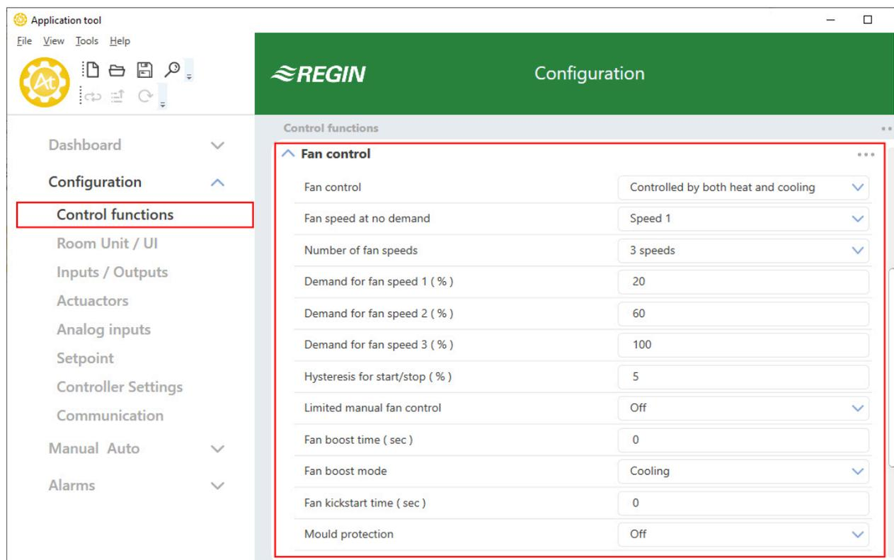
Figure 3-34 3-speed fan control configuration settings in Application tool.
