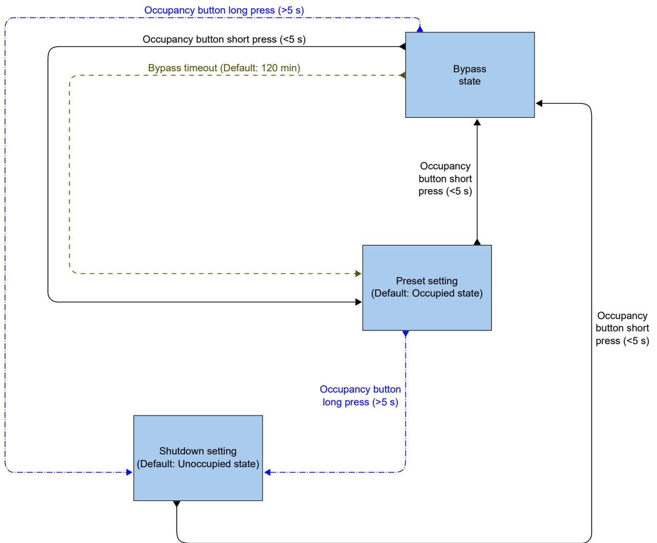
Figure 3-29 Flow chart describing controller state changes for when the occupancy (on/off) button on the controller is used.
