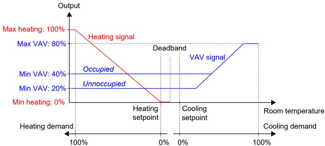
Figure 3-39 VAV control behaviour based on cooling demand when a maximum limit is set, and minimum limits for the occupied and unoccupied controller states are set.
