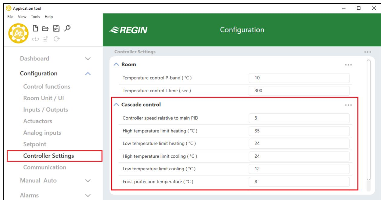
Figure 3-47 Cascade control configuration settings in Application tool.
