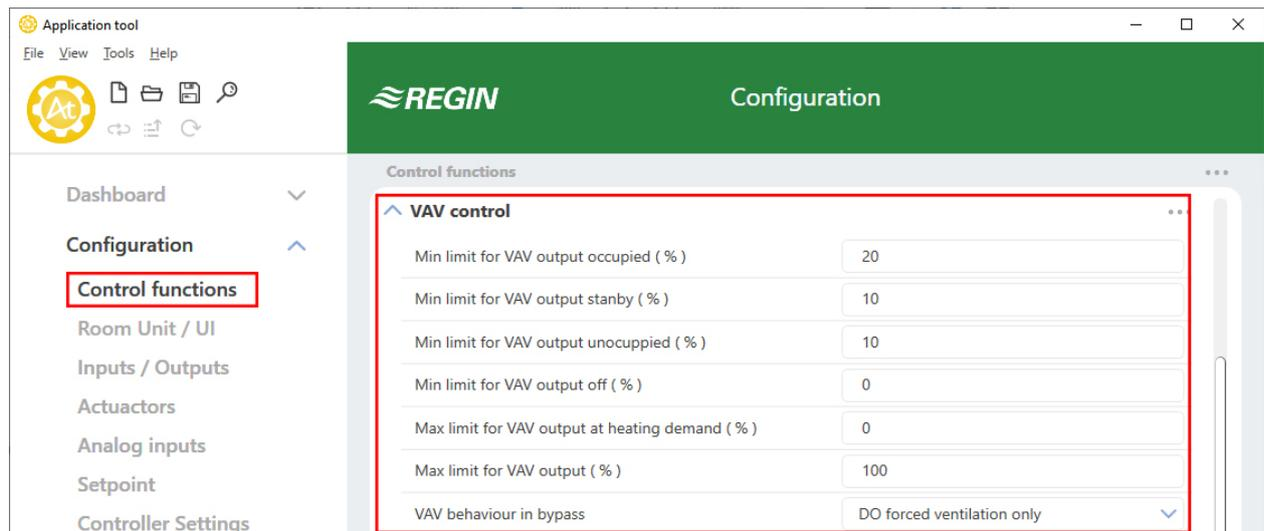
Figure 3-38 VAV control configuration settings in Application tool.
