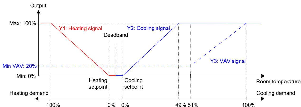
Figure 3-11 Control behaviour for the Heating + Cooling + VAV controller mode when the controller regulates based on heating and cooling demand.
