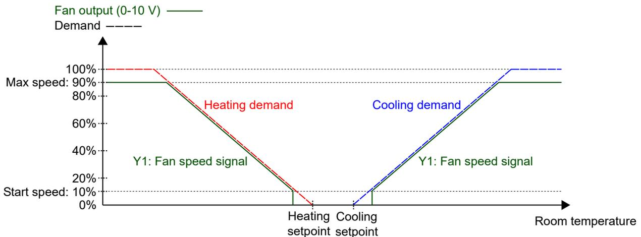
Figure 3-32 EC fan control behaviour in auto mode.
