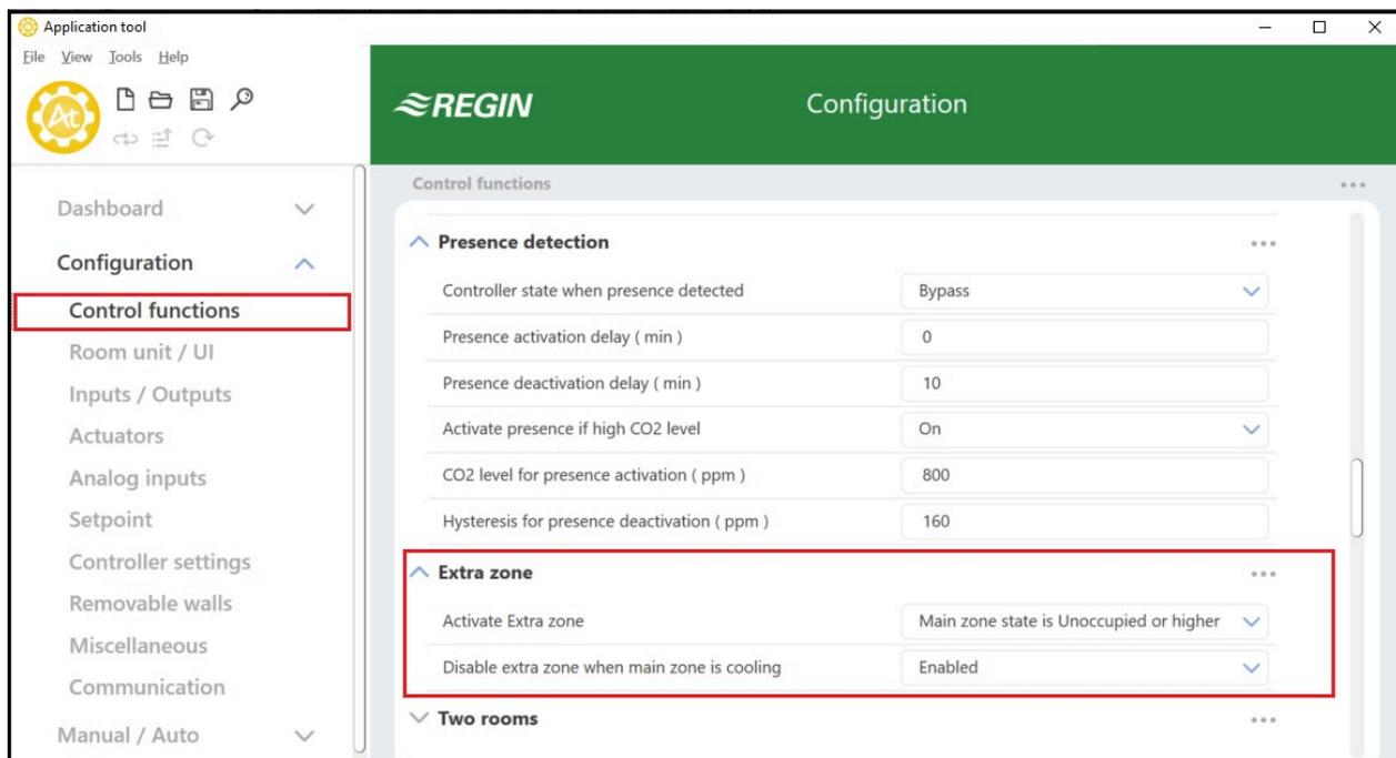
Figure 3-46 Extra zone configuration settings in Application tool.
