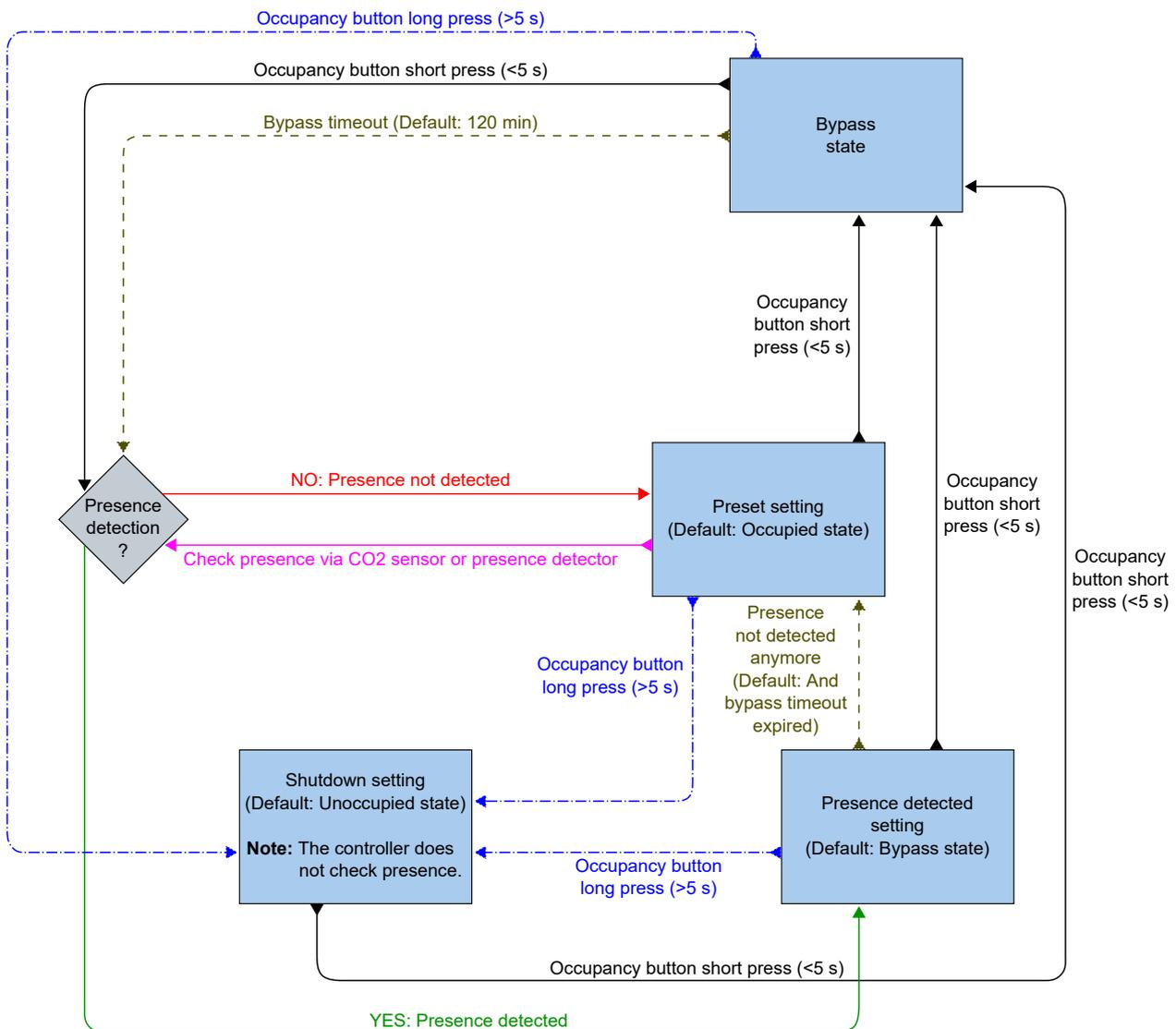
Figure 3-30 Flow chart describing controller state changes for when presence detection and the occupancy (on/off) button on the controller is used.
