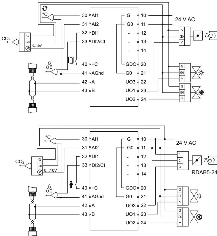
Figure 6-3 Connection diagrams for model for CO<sub>2</sub> control.
