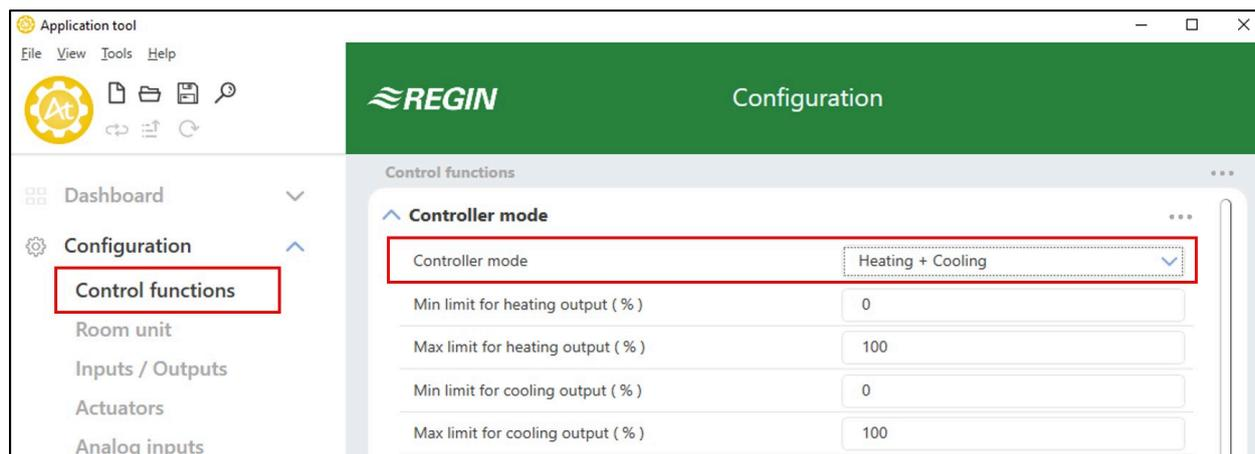
Figure 3-1 Controller mode selection in Application tool.
